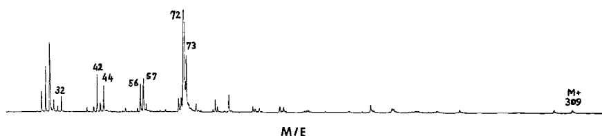
FIG. 2—Mass spectrum of methadone.
