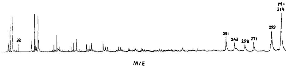
FIG. 3—Mass spectrum of tetrahydrocannabinol.
